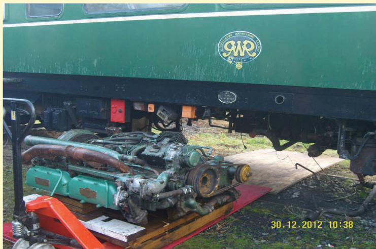
Engines being refitted to 52062, 30/12/12 (K.Jones)
