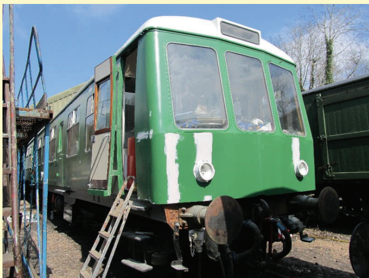
The filling work on the front end after a new one was fitted, 20/4/13
