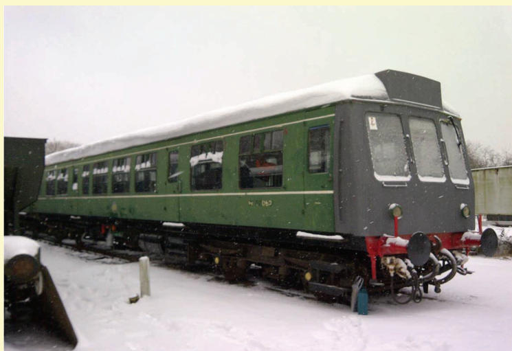
52062 after cab bodywork repairs (K.Jones)
